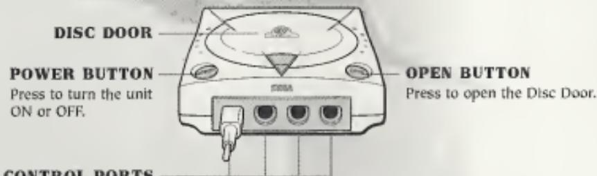
Use these ports to connect the Sega Dreamcast™ Controller or other peripheral equipment. From left to right are Control Port A, Control Port B, Control Port C, and Control Port D. For **CAPCOM VS SNK MILLENNIUM FIGHT 2000**, use Control Ports A and B to connect controllers for players 1 and 2 respectively.
