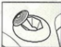
SI LA MANETTE EST EN POSITION **INCLINÉE** (COMME ILLUSTRE SUR LE DESSIN DE GAUCHE) AU MOMENT OÙ ELLE EST MISE SOUS TENSION, CETTE POSITION SERA RÉGLÉE COMME LA POSITION NEUTRE. LES CONTRÔLES SERONT FAUSSES PENDANT LA PARTIE.
