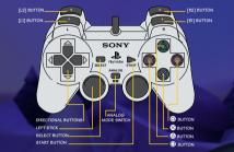
Note: DUALSHOCKT# analog controller only: Toggle the vibration function ON/OFF by using the Options mode Vibration setting. The Vibration setting is not affected by the controller's analog mode switch.
